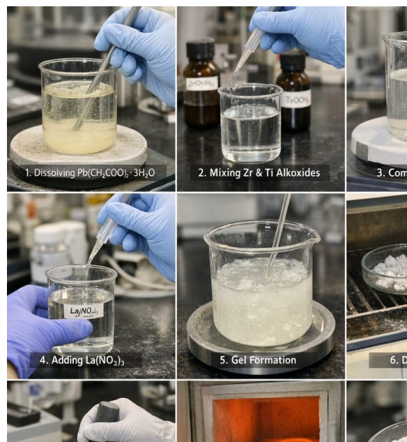
Fig. 1. Step-by-step photographic representation of the Sol-gel synthesis of PZT/La-doped PZT
